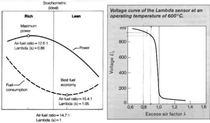
The output of the Lambda O2 sensor is a voltage as shown in the graph on the above right. So, all we have to do is connect the sensor to a voltmeter and we're set, right? Wrong! The sensor voltage source is high impedance, which means it can't deliver much current or power. This voltage can only be measured accurately after power amplification. Electronic test instruments (which contain power amplification) be used to accurately measure the voltage, but the
