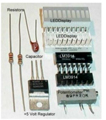
My first display circuit had a linear output; the first LED turned on at 0.09V, the second at 0.18V, the third at 0.27V and the last (tenth) at 0.90V. I used the bar graph mode so that the LEDs turned on at a lower voltage stayed on when addition LEDs were turned on. When the last LED turned on at a voltage grater than 0.9V, all the LEDs were on.
